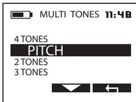
Pitch mode is completely different from the others. It does not take into account the target's conductivity: the strength of the signal generates an audio signal that varies both in amplitude and height (the audio frequency). This means that a more distant target will generate a low-pitched, weak sound whereas a closer target will generate a high-pitched, strong sound. Pitch mode gives signals particular "characteristics" and can be useful for locating targets.
