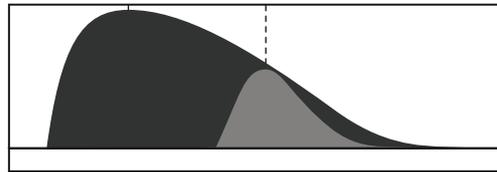
With a low Reactivity level, the iron is detected for a longer duration, to the extent that it completely hides the ring.
