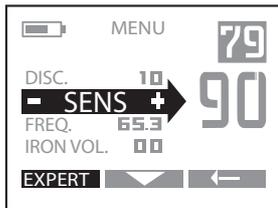
Dēus enables you to adjust the strength of the emitted electromagnetic field according to three levels (from 1 to 3).
