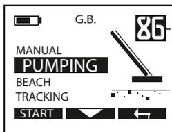
**Non-motion Audio Disc** and **Non-motion All Metal** require an adjustment of the ground balance. Pump the coil to the ground (refer to explanation on page 17) and manually adjust the ground setting on the value displayed at the top of the Ground Balance screen.
