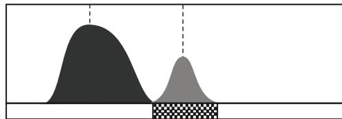
A high Reactivity level enables you to distinguish the ring completely from the iron. The audio signal fully indicates the target.
