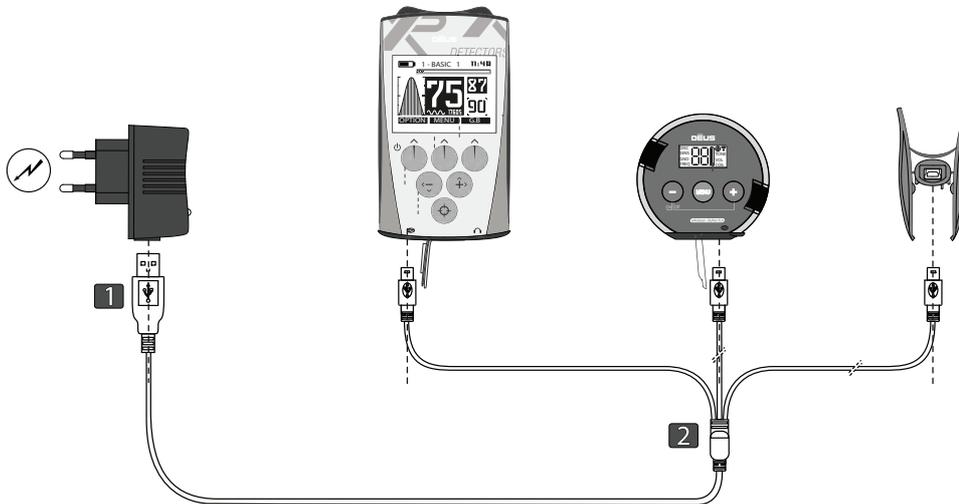
The search coil is charged via the connection clamp supplied, which is connected to the coil according to the grooves in the coil cover.
