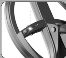
The LED on the coil gives 20 long, successive flashes to indicate that it is waking up and recalibrating.
