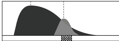
With a medium Reactivity level, you begin detecting the ring. The audio signal partially indicates the target.
